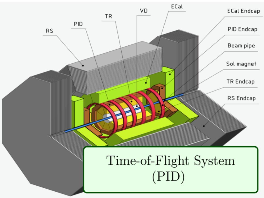
Time-of-Flight System (PID)
