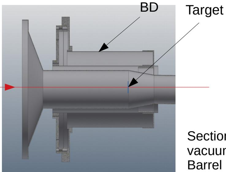
Section of carbon vacuum pipe and Barrel Detector
