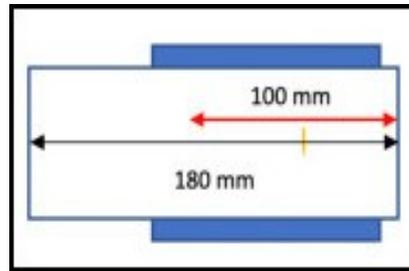
Inner shield (5mm thick)
