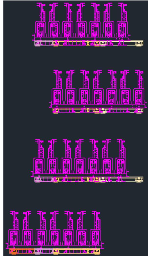
Stages of changing the mechanical support for GEM detectors, taking into account the future stages of modernization of the central tracking system of the BM@N setup
