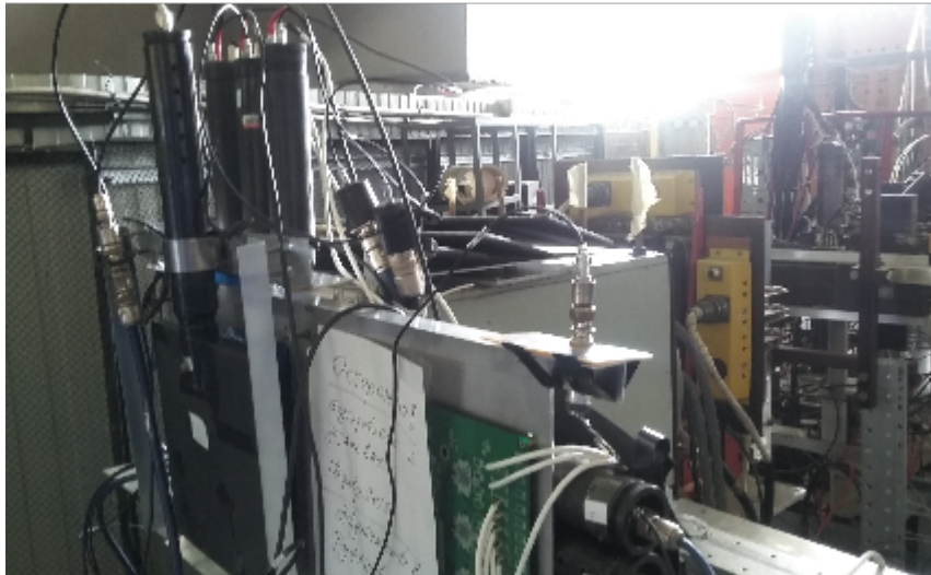
A general view of ECal based on BGO crystals with veto-detectors at NIS-GIBS setup, 2015 (Nuclotron, JINR)
