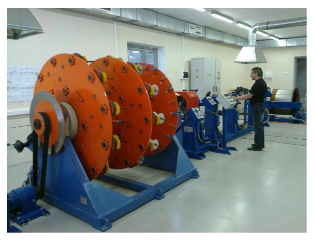
Machine for production Nuclotron-type superconducting cable
