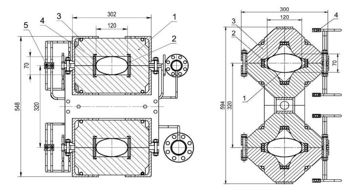
Cross-section of the collider magnets: Dipole magnet (left): 1 – lamination, 2 – SC coil, 3 – tube for cooling the yoke, 4 – beam pipe, 5 – bus bars; Quadrupole lens (right): 1 – beam pipe, 2 – half-yoke, 3 – lamination, 4 – bus bars. All dimensions in mm.
