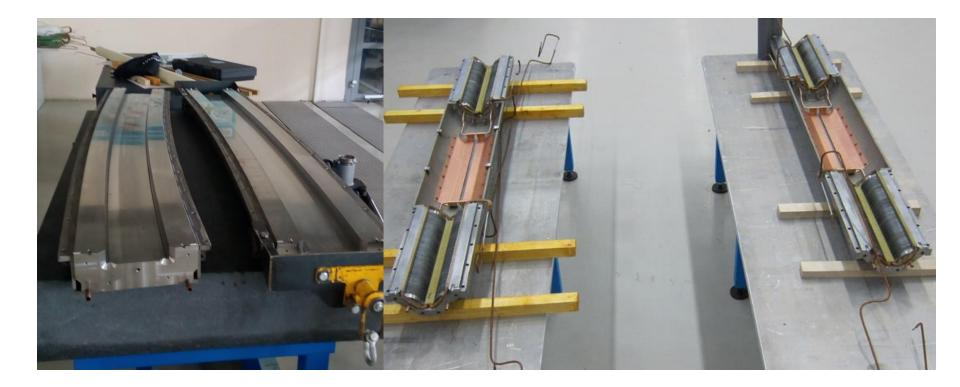
Half-coils assembling with half-yokes for the booster dipole magnet (left) and doublet of the lenses (right)
