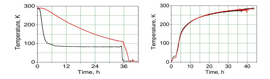
Cooling-down (left) and warm-up (right) of the dipole magnet for the NICA booster. Black line is inlet and red line – outlet of the magnet.
