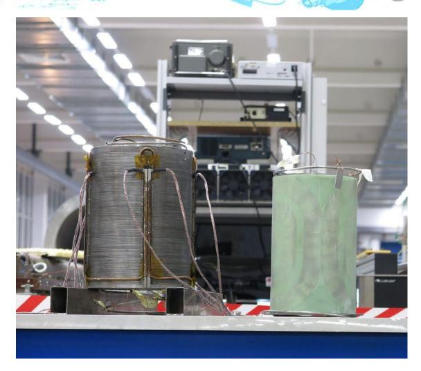
24 steering magnets will have two coils each (horizontal and vertical dipole coils) and 8 corrector magnets will contain four coils each (normal and skew quadrupole and sextupole coils).
