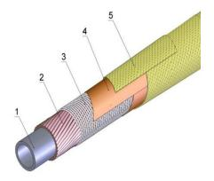
View of Nuclotron-type cable: 1 - cooling tube, 2 - SC wire, 3 - Ni-Cr wire, 4 and 5 - insulation
