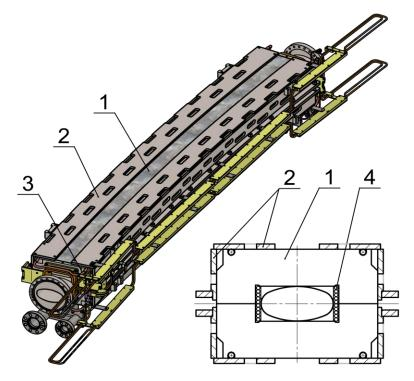
View of the dipole magnet. 1 – lamination, 2 - side plate, 3 - end plate, 4 – SC coil.
