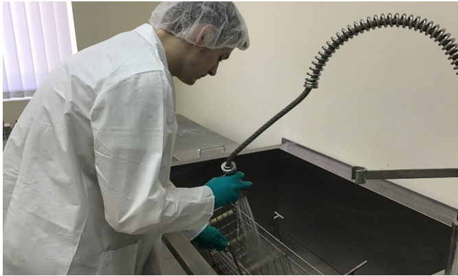
Glass cleaning with ultrasonic wave & deionized water
