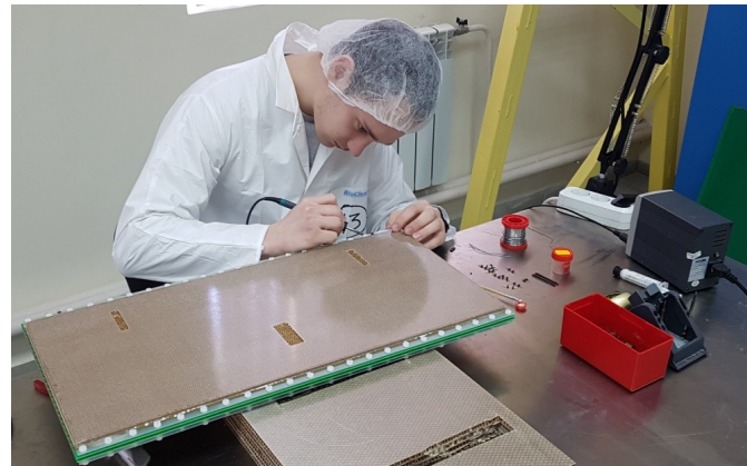
Soldering HV connector and readout pins
