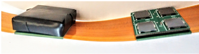
FIG. 4: General front-end PCB prototype. The picture shows the the SFED card attached to the ribbon card.
