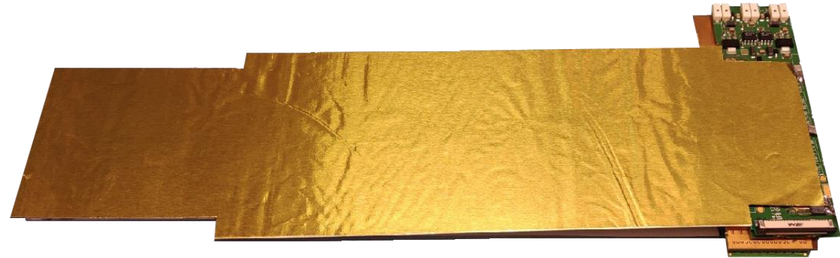
Assembled module covered with shieldings (JINR)
