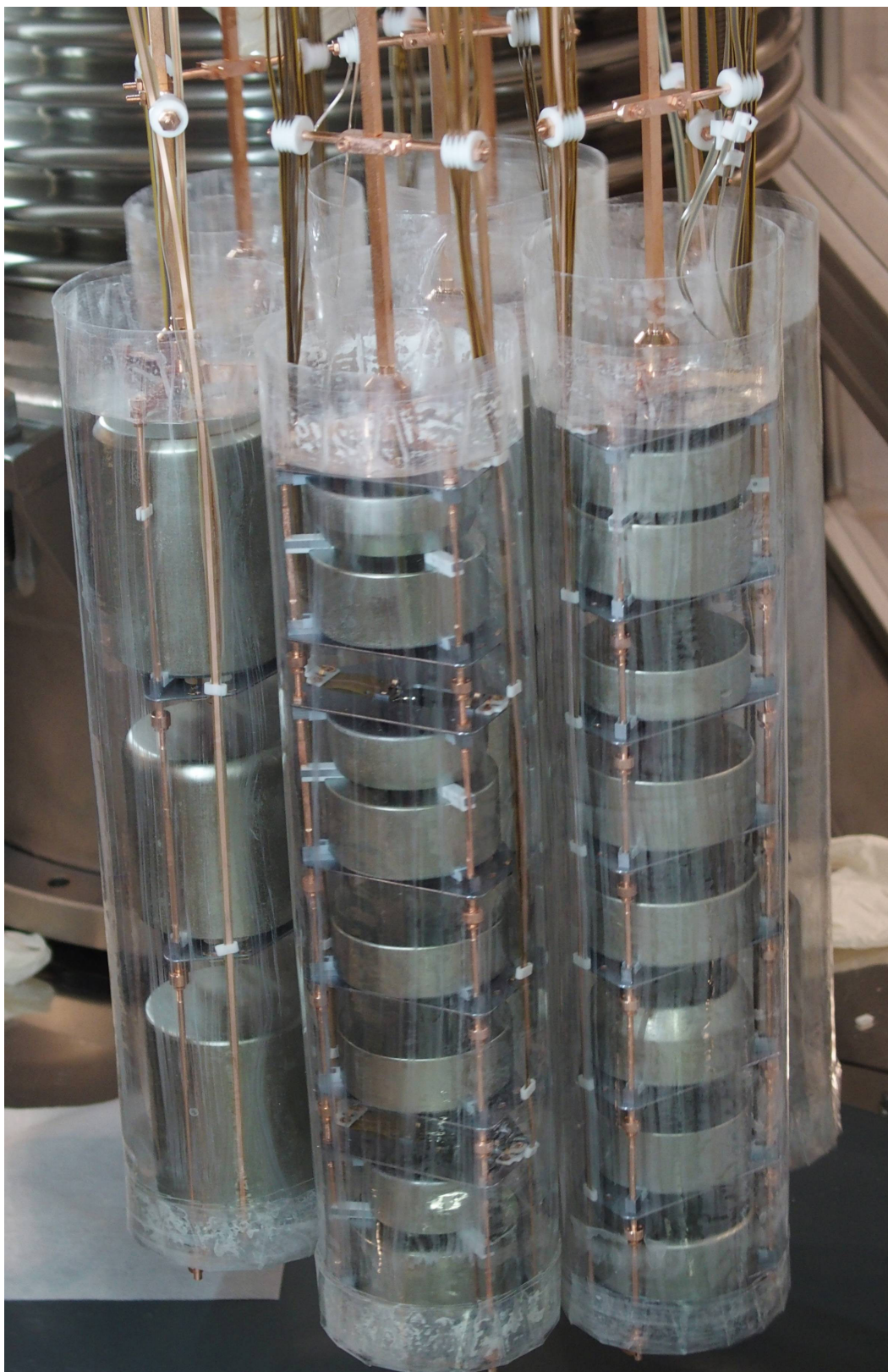
Extended Data Figure 3 | Germanium detector array. Photograph of the assembled detector array, with a string of coaxial detectors on the left, and strings of BEGe detectors at middle and right. Each string is enclosed by a cylindrical nylon shroud covered with a wavelength shifter.
