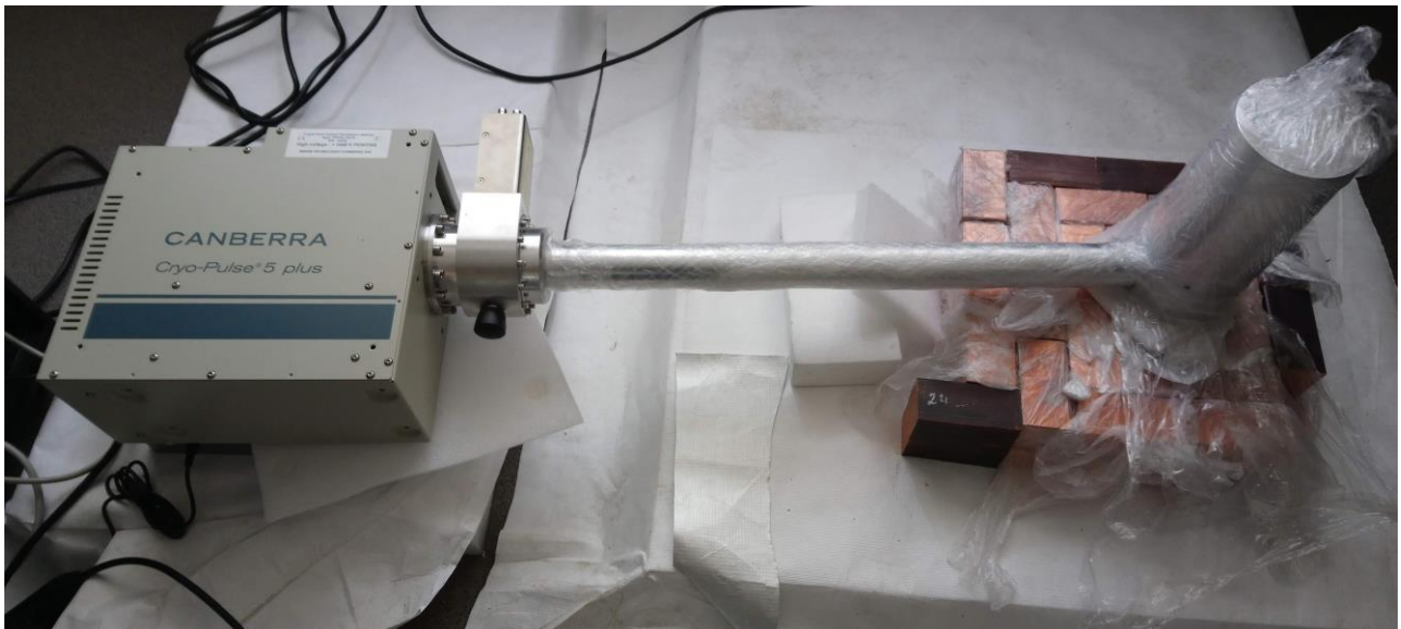
Figure 3. Photo of one HPGe point contact vGeN detectors with electric cooling.
