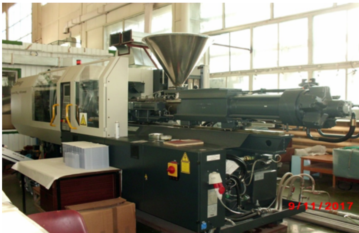
Figure 4.13: The scintillator production facility: moulding machine.
