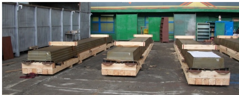
Fig. 2.2.1.13. Forgings of beams at NKMZ before shipment.
