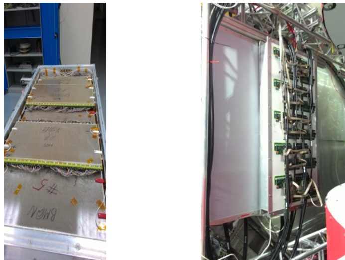
Fig. 2.2.2.53 Gas box (module) with packed detectors (left) and a left part of ToF-400 wall mounted in BM@N hall (right).
