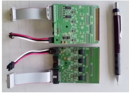
Fig. 2.2.2.43. 128 channel read-out board. Front and back side view.
