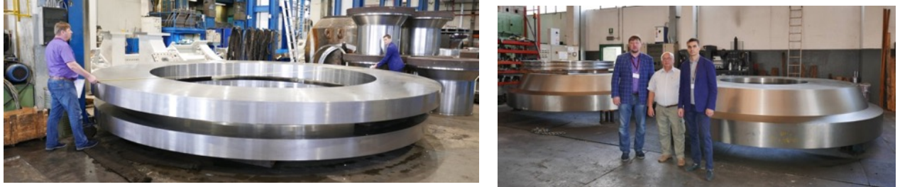
Fig. 2.2.1.14. Forgings of support rings and poles after preliminary processing with an allowance of 5 mm per contour (June 2016).
