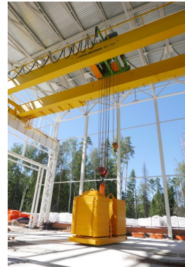
Fig. 2.3.5.1. Installation and testing of booster crane beams, May 2016 (left) and static tests of crane with lifting capacity of 80 tons. The weight of the control load is 100 tons, June 2019 (right).
