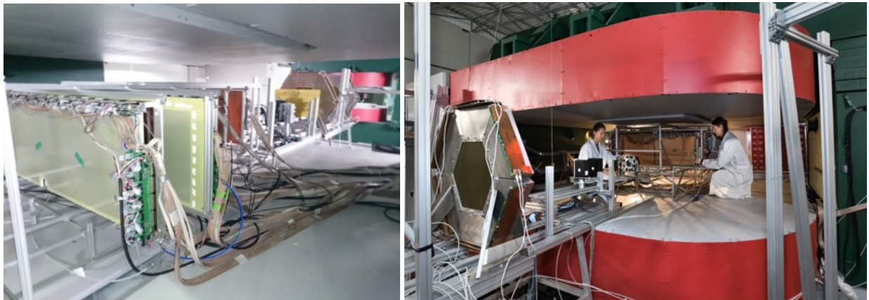
Fig. 2.2.2.34. GEM chambers integrated into BM@N experimental setup
