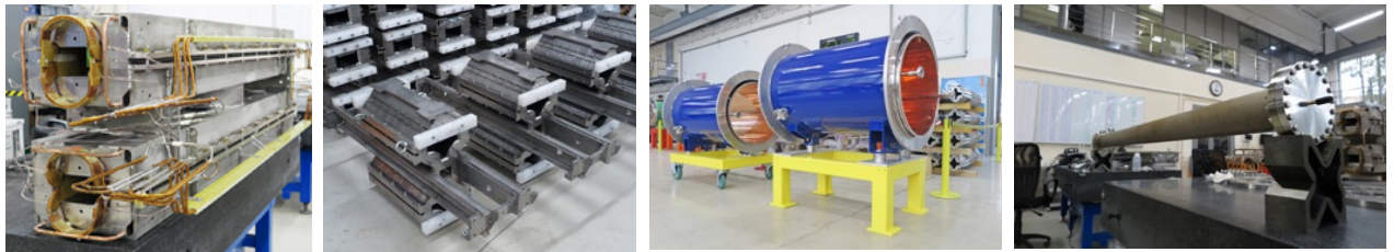
Fig. 2.1.5.1. From left to right: dipole magnet, quadrupole lenses, cryostats and vacuum beam pipe of the Collider.
