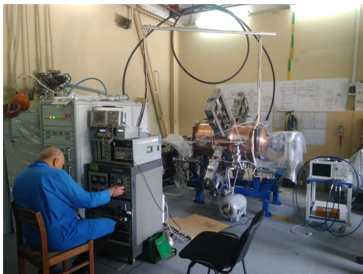
Fig.2.1.5.6 Test of working RF-2 prototype station.
