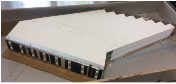
Fig. 2.2.1.47. Prototype modules. On the bottom-left panel, the readout electronics board is shown.
