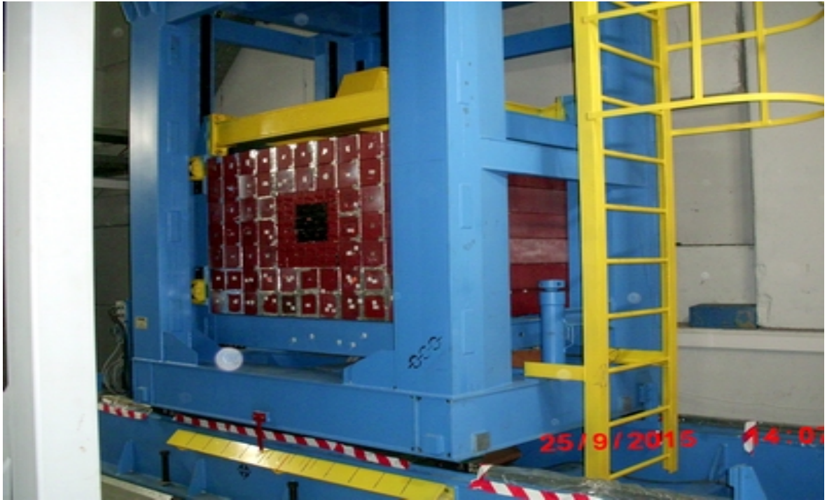
Fig. 2.2.2.65. ZDC from 104 modules completely assembled.
