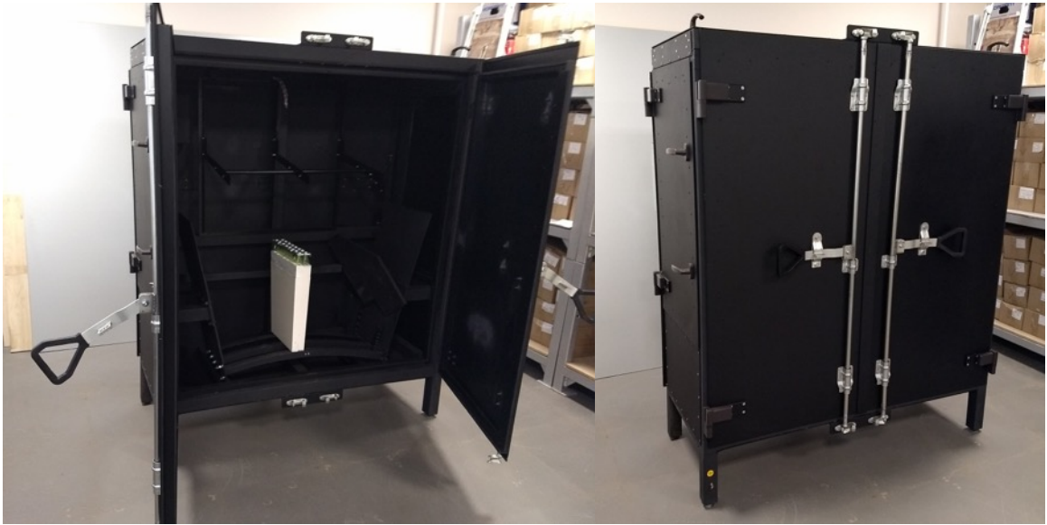
Fig. 2.2.1.52. Prototype stand to test simultaneously 12 Ecal modules in one load with cosmic muons.
