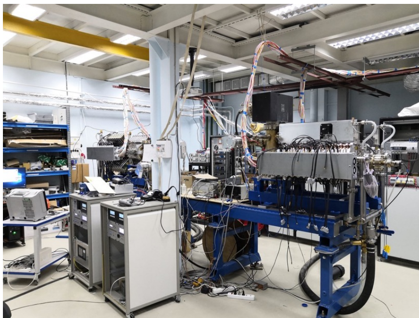
Fig. 2.1.5.3. RF-1 voltage station.
