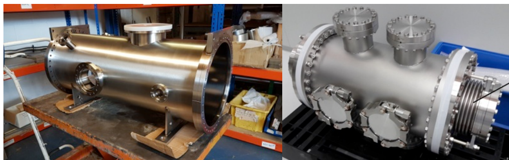
Fig. 2.1.3.11. Electrostatic septum during manufacturing (left) and inflector plates IP2 (right).
