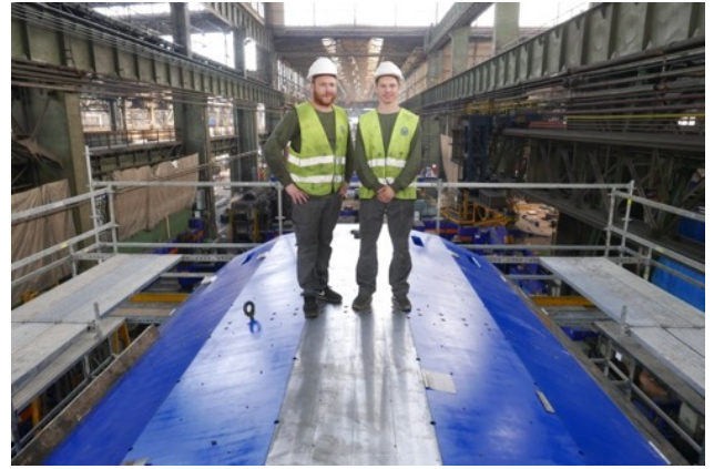
Fig. 2.2.1.15. Installing the first bottom plate of the magnetic circuit (left). The magnetic circuit is assembled. June 2018.
