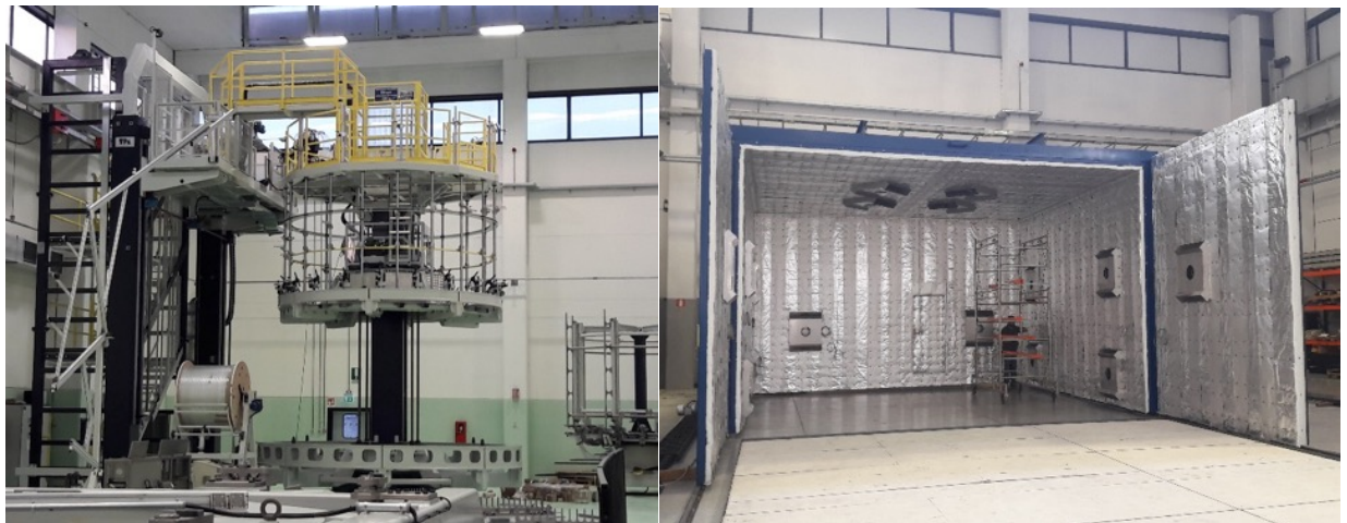
Fig. 2.2.1.6. Winding machine (left) and “impregnation” oven (right).
