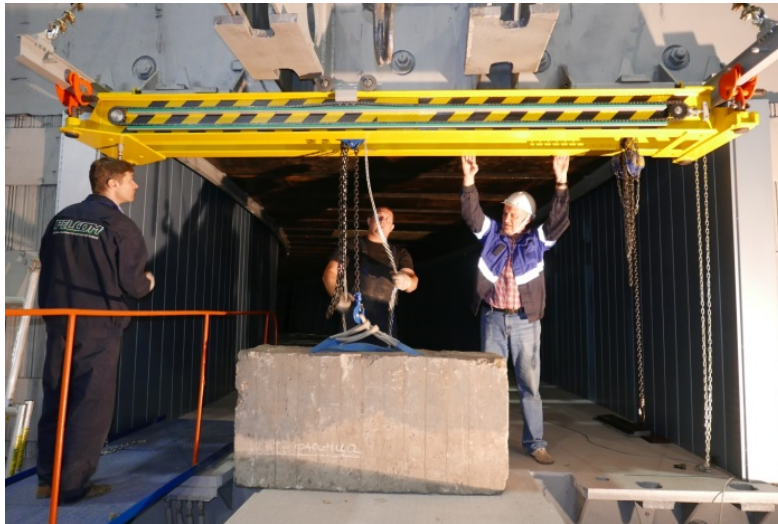
Fig. 2.3.5.1. Installation and testing of booster crane beams, May 2016 (left) and static tests of crane with lifting capacity of 80 tons. The weight of the control load is 100 tons, June 2019 (right).
