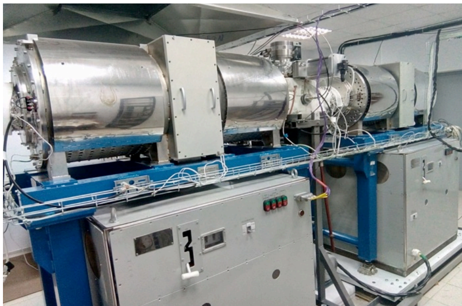
Fig. 2.1.3.20. The Booster accelerating stations at JINR test bench
