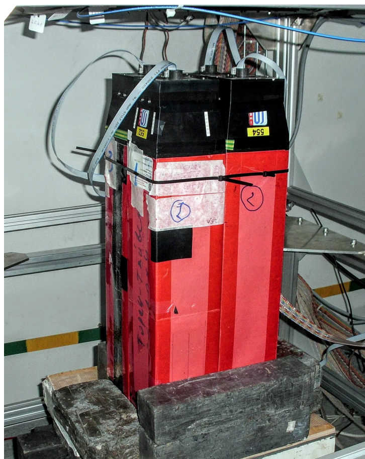
Figure 4.17: Photo of the calorimeter test setup, consisting of 4 modules of size 11 \times 11 \text{ cm}^2 , with total cross section of 22 \times 22 \text{ cm}^2 .
