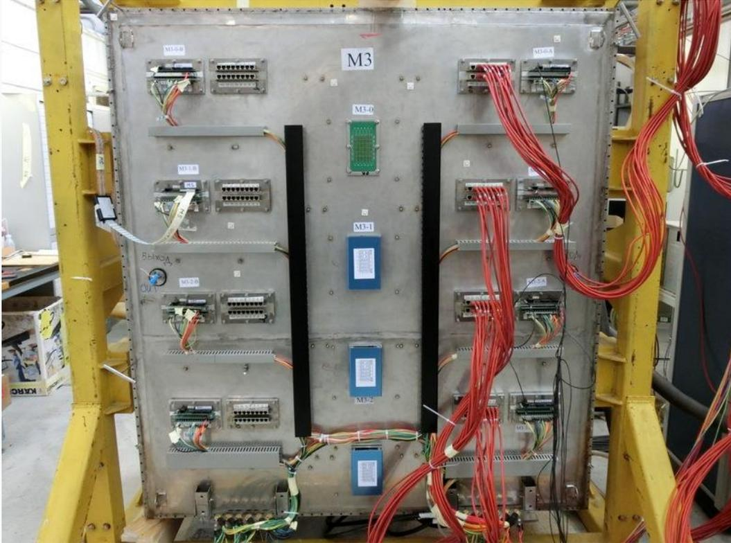
Figure: 9. Module with closed lid. All connections to the cards from the outside made through sealed flanges.
