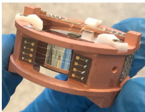
Fig 5.2: Photograph of a 10 mm height and 30 mm diameter Ge detector prototype with 4 electrodes, one NTD-Ge heat sensor mounted in its copper holder. Right: Neutron calibration of the detector represented on the quenching versus recoil energy. Two populations of events are: electronic recoils with Q \sim 1 (red band) and nuclear recoils with Q \sim 0.3 (blue band). Electronic captures from the K and L shells of the ^{73}\text{Ge} at 10.37 keV and 1.3 keV respectively are also visible and are used for calibration. Those two lines have been activated by an exposition of the detectors to a high activity neutron source.
