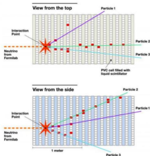
Liquid-scintillator detectors have segmented structure.
