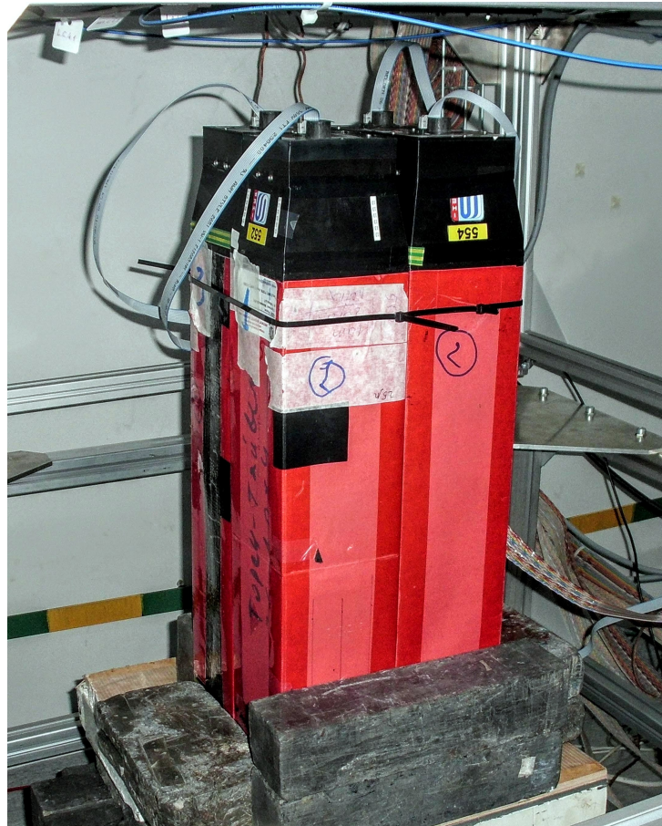
Figure 4.21: Photo of the calorimeter test setup consisting of 4 modules of the size 11 \times 11 \text{ cm}^2 , with the total cross-section of 22 \times 22 \text{ cm}^2 .
