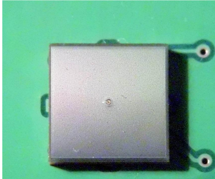
SiPm 6x6mm 2 with pixel size of 25 micron
