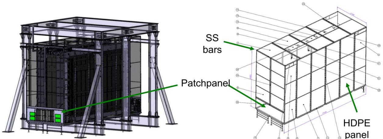
**Figure 7.** Final design of the anti-radon tent.
