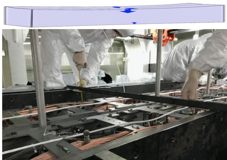
**Figure 9.** Top: the nature of the sagging of the track chamber. Bottom: methodological studies (measurements) of the sagging at the LSM.
