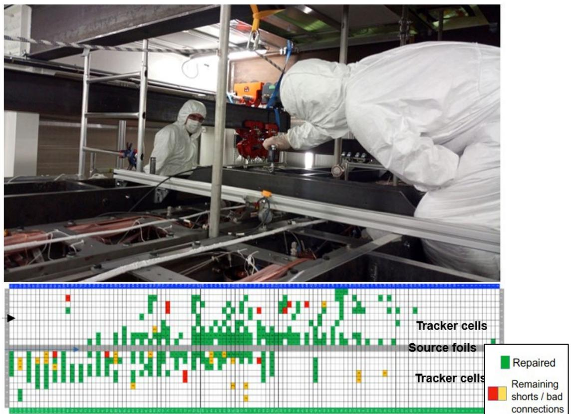
**Figure 10.** Top: lifting of the top of the tracker. Bottom: map of the restored Geiger cells.
