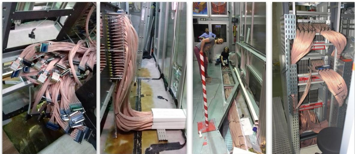
**Figure 6.** Cabling up of the tracking detector of the SuperNEMO Demonstrator.
