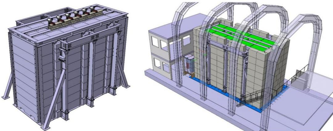
**Figure 9.** The structure of iron shielding (left) and its integration with neutron shielding (borated polyethylene) in the underground laboratory.
