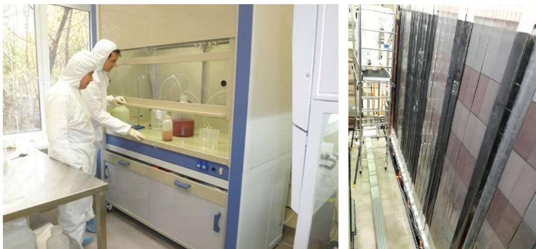
**Figure 3.** Left: clean room created at the JINR DLNP for radiochemical purification of isotopes (Se-82). Right: Se-82 source foils installed inside SuperNEMO Demonstrator.
