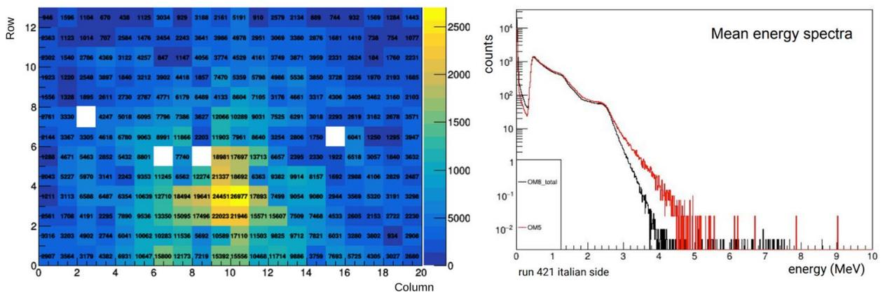
**Figure 11.** Counting rate of optical modules in a run with Co-60 source for one of the calorimeter walls (left). Energy spectra of all 5-inches and 8-inches optical modules (right).
