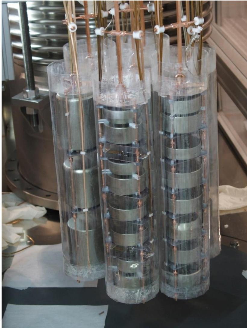
The NMS for GERDA Phase II were made from nylon. Nylon pieces were covered by WLS and formed to NMS with a clean glue.
