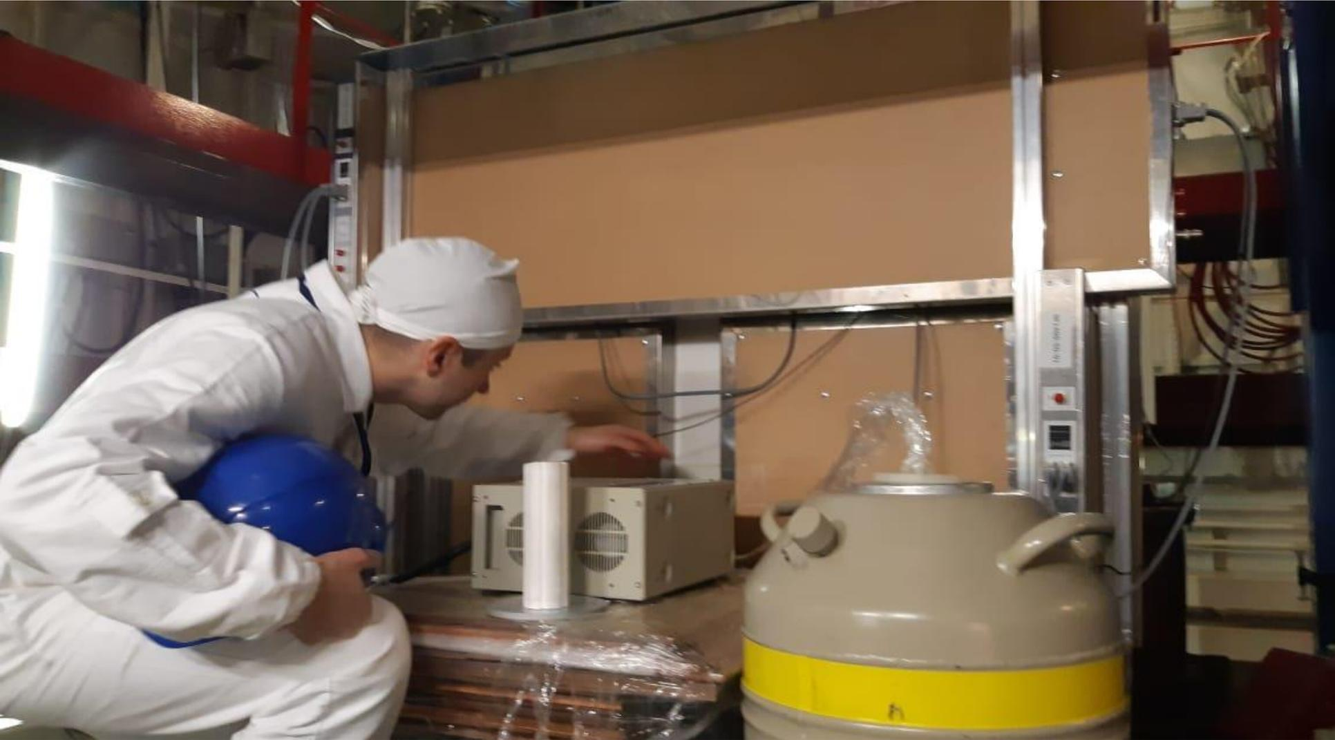
Nitrogen flushing is used to suppressed radon background.
