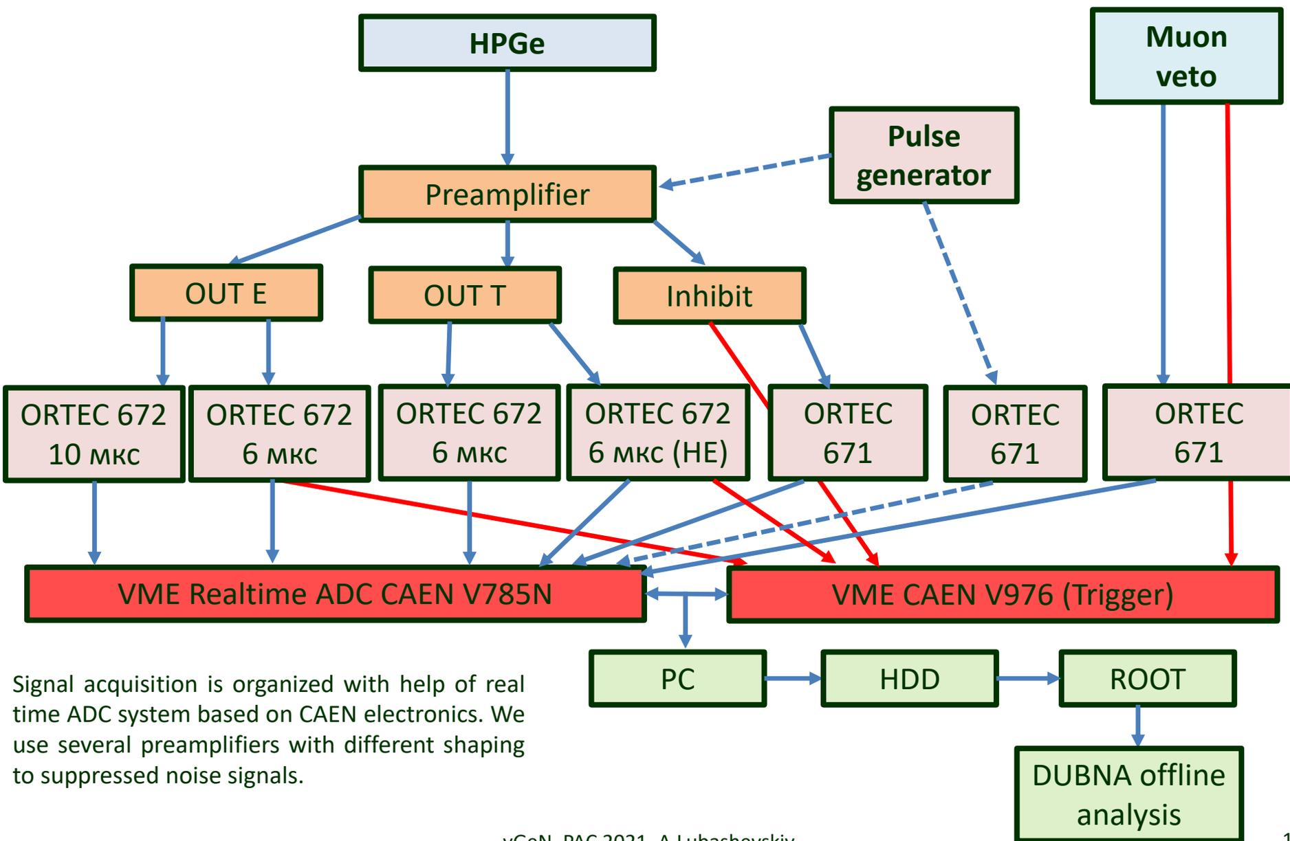
Signal acquisition is organized with help of real time ADC system based on CAEN electronics. We use several preamplifiers with different shaping to suppressed noise signals.
