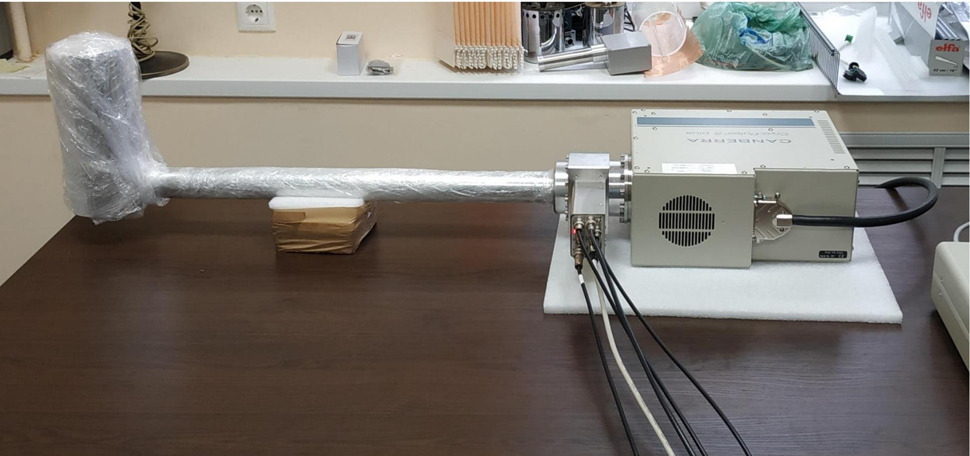
To detect signal from neutrino scattering we use specially produced by CANBERRA (Mirion, Lingosheim) low-threshold, low-background HPGe detectors. We use detectors both with electric and nitrogen cooling.
