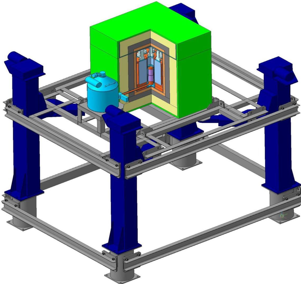
We produced a special lifting mechanism to move the spectrometer towards the reactor core to change the neutrino flux through the detector. Such device also helps to distinguish neutrino signals from the background.
