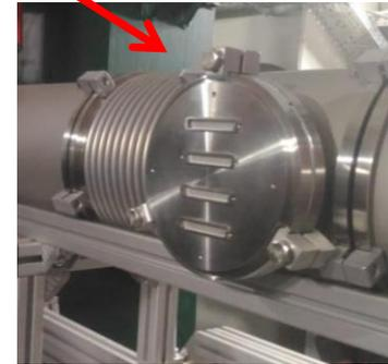
Four stainless steel vacuum boxes downstream the target are replaced by aluminum ones. The design and production of the target station pneumatic actuator mechanics is performed by A.Kubankin group.
