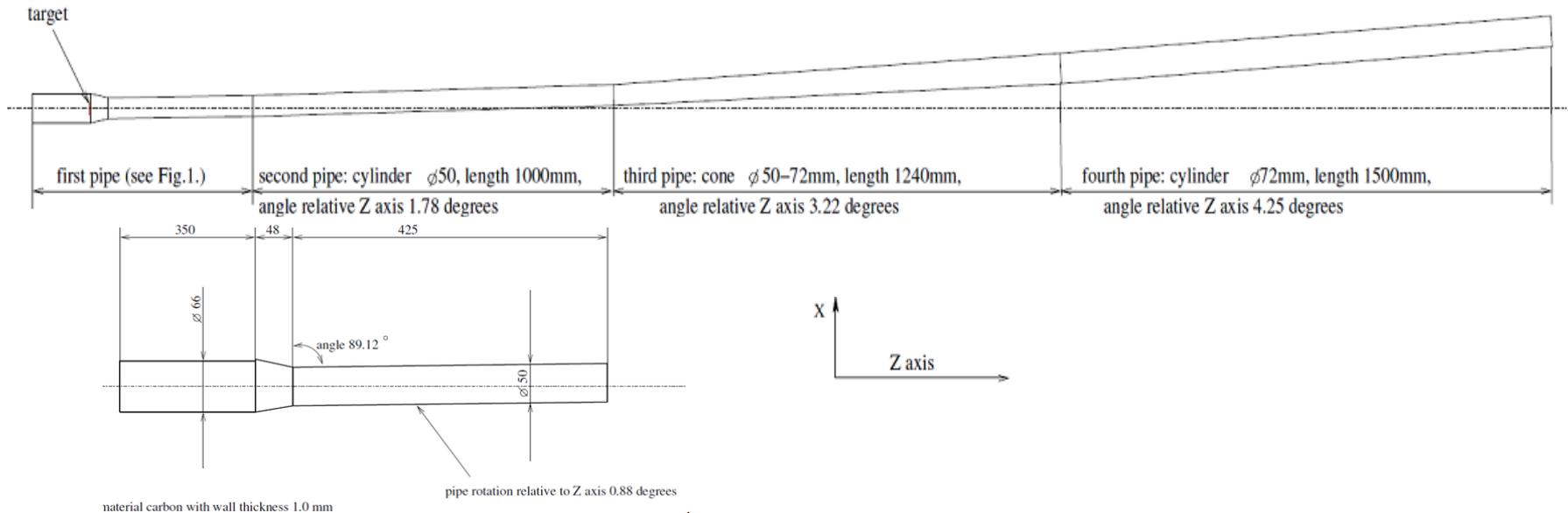
**BM@N carbon beam pipe configuration (Au 3.8 AGeV 1800 A ~ 0.9 Tl)**
