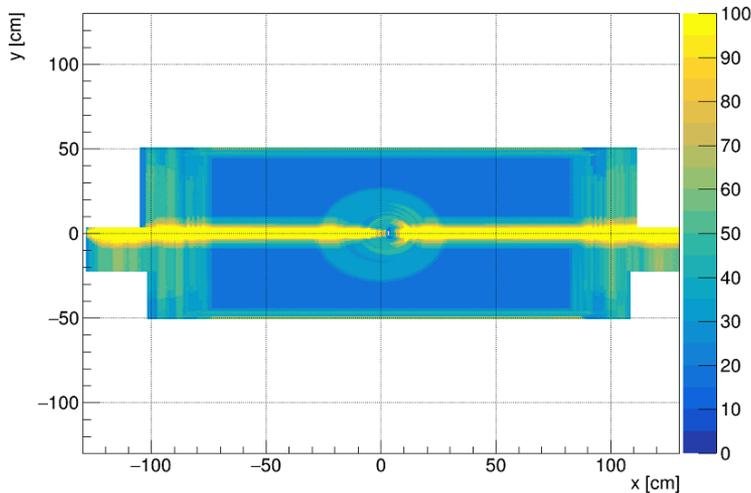
Material budget in the BM@N, Integrated radiation length,  $X/X_0$  [%]
