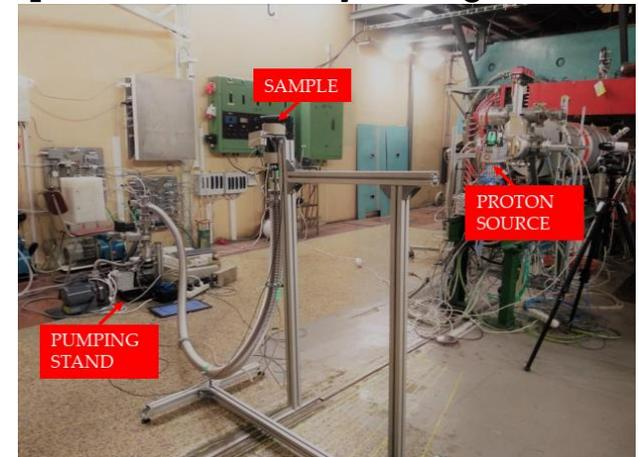
The ultimate pressure  $6 \times 10^{-6}$  hPa (scroll pump and turbomolecular pump)
