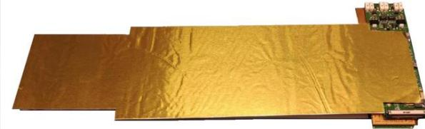
Assembled module covered with shielding
