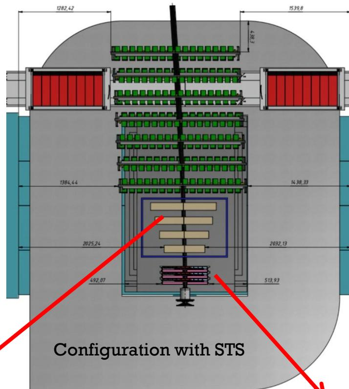
Forward Si will be removed after integration of STS full configuration into BM@N setup (after 2022 year, high beam intensity - few  $10^6$  Hz)
