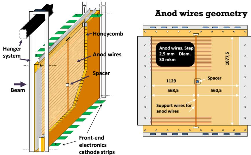
Design of the 1065x1065 mm<sup>2</sup> CSC chamber
