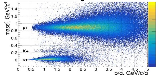
Preliminary result of identification, GEM+DCH track extrapolated to ToF-700
