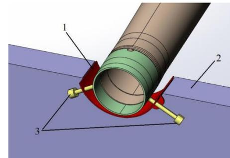
Design of the support system, which uses the surface of GEMs
