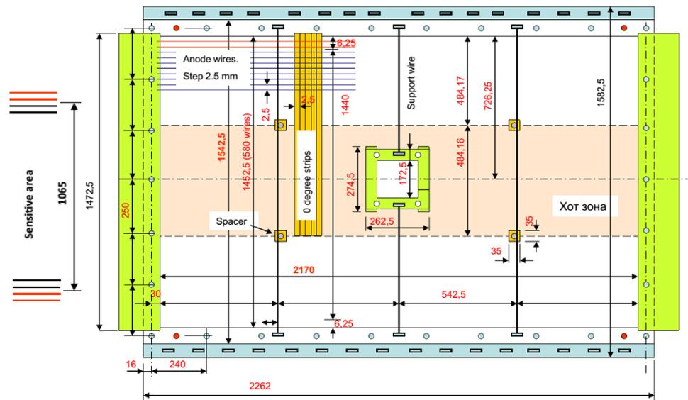
Design of the 2190x1453 mm<sup>2</sup> CSC chamber
