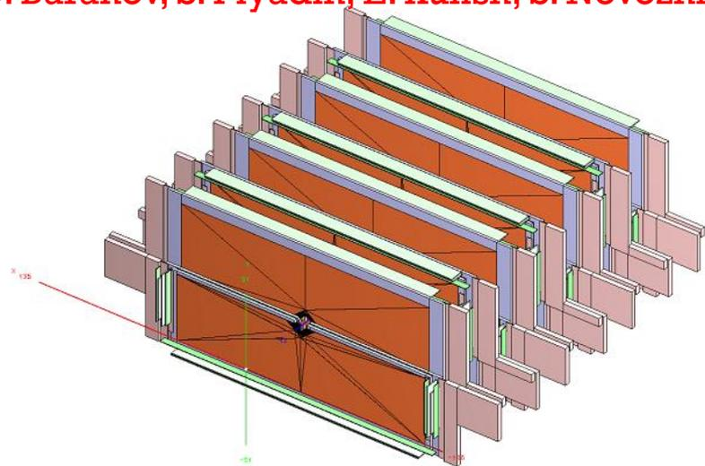
Detailed geometry of GEM planes for heavy ion beam runs (Left panel: GEM active areas, right panel: mechanical support frames and FEE electronics are added )
