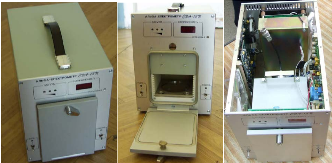
Fig. 9.5: Photo of the vacuum chamber of the alpha spectrometer containing electronic module (preamplifier, shaping amplifier, power supply, vacuum control module).
