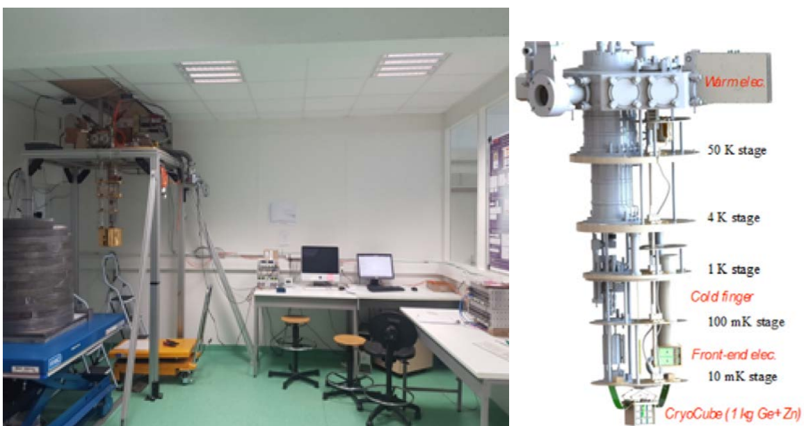
Fig. 9.4: Left: Test EDELWEISS/Ricochet dry cryostat. Right: Scheme of the Ricochet cryostat.
