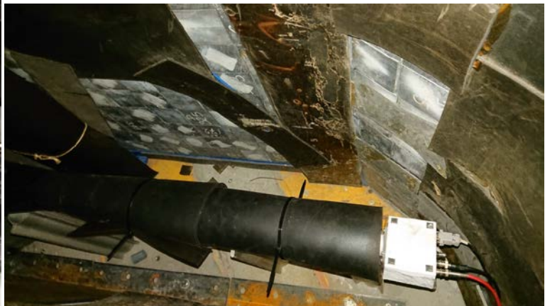
Fig. 9.2: Photo of the ^3\text{He} filled proportional counter installed at close proximity to the EDELWEISS cryostat (left) and at ILL Ricochet site (right).
