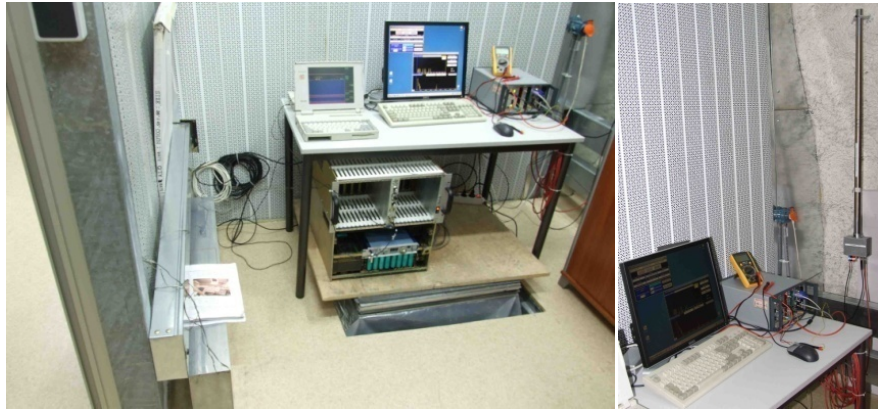
Fig. 9.1: Detectors developed at JINR for study of neutron background at EDELWEISS environment. Left picture is detector of fast neutrons; right one is detector of thermal neutrons (on the wall).
