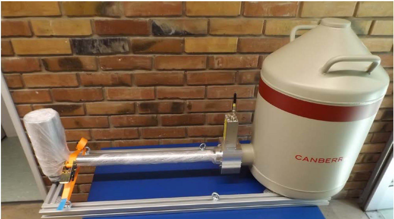
Figure 2. Photo of one HPGe point contact vGeN detectors.
