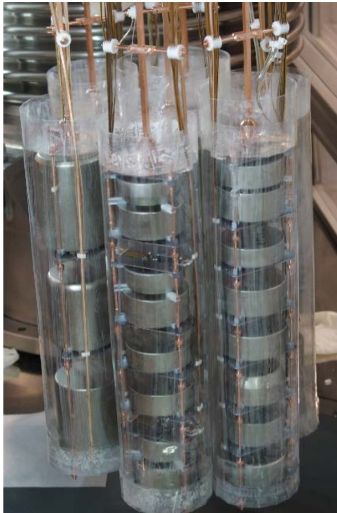
Fig. 13. Photo of GERDA Phase II detector array. Each of the seven strings is enclosed by a transparent mini-shroud.
