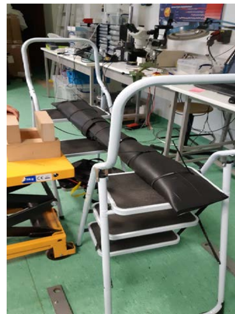
Figure 3.6: Photography of both He3 detectors in the lead shielding used for the cryostat.
