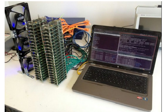
A 42-node cluster of Parallella-16 boards from Adapteva
