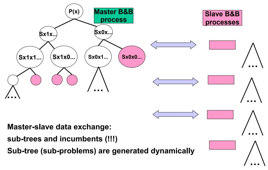
Usually, the approach is based on MPI and run at high-performance cluster
