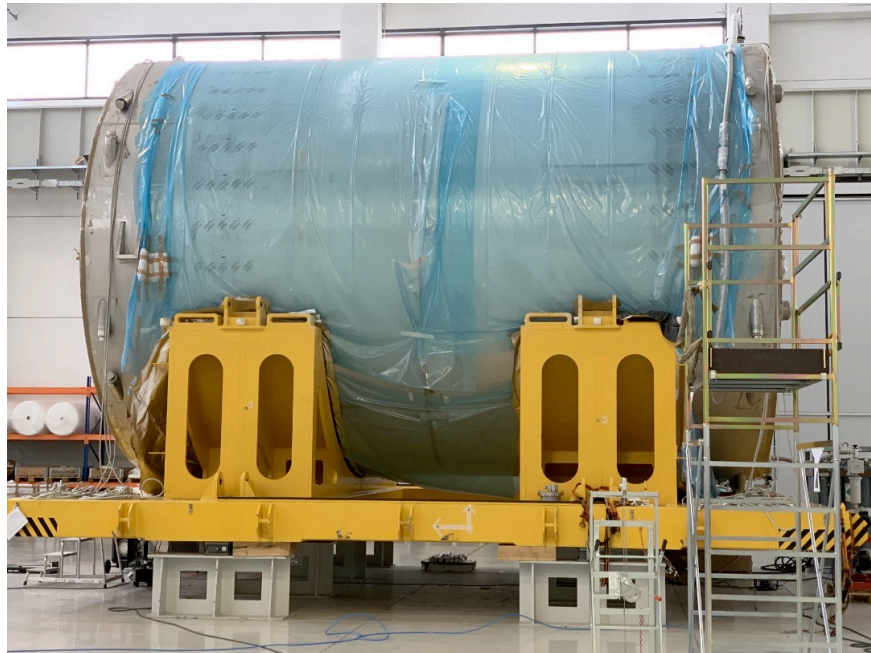
Fig.3.2.2 . Completely built solenoid.
