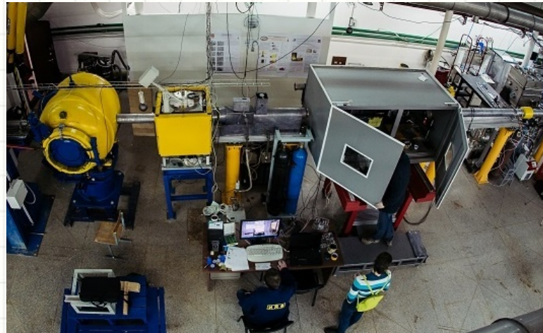
High-speed temporal radiography of detonation processes
