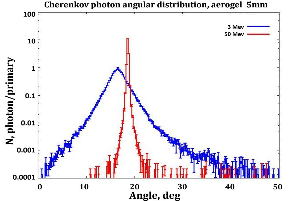
The angular distributions of Cherenkov photons emitted by **3 MeV** and **50 MeV** electron beam passing through 5mm of a quartz aerogel.
