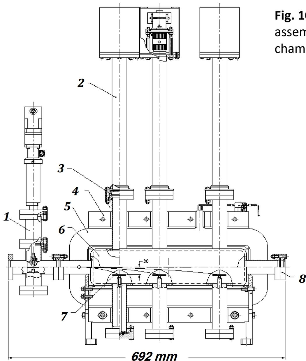
**Fig. 10.** Layout of spectrometer: 1 - collimator, 2 - digital camera assembly, 3 -vacuum window, 4 - magnetic core, 5 - coils, 6 - vacuum chamber, 7 - plate with applied phosphor, 8 –Ti outlet window.
