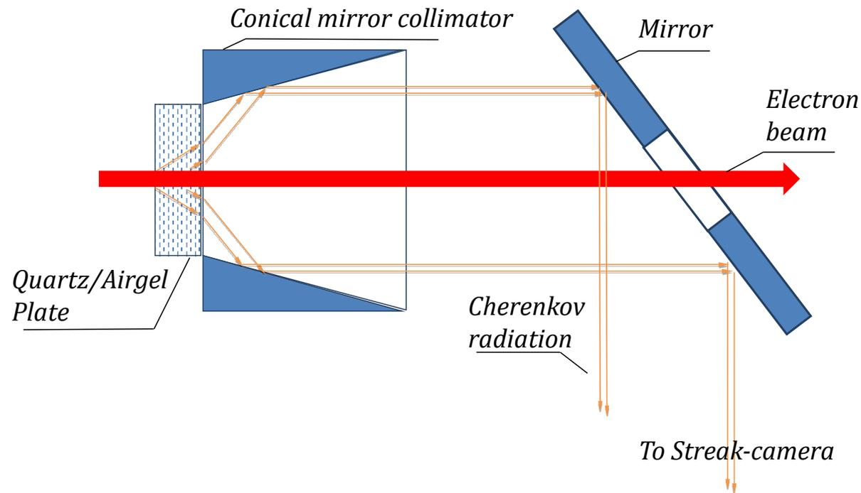
**Layout of Cherenkov sensor for measuring longitudinal bunch profile.** Cherenkov radiator is manufactured from quartz for beam energy  $E = 0.6$  MeV and from quartz aerogel for  $E = 3$  MeV and higher.
