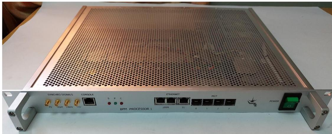
**Fig. 5.** BPM Processor module from the BINP
