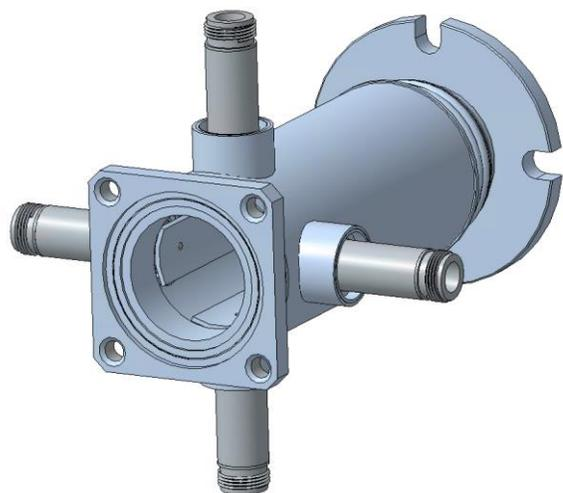
2. Button type BPMs with button diameter of 15 mm (Booster)
