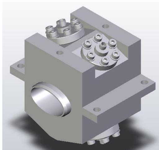
3. Button type BPMs with button diameter of 6 mm (Storage ring)
