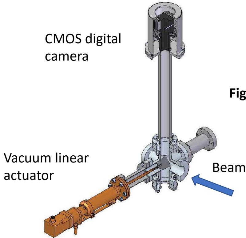
**Fig.8.** Layout of scintillating screens
