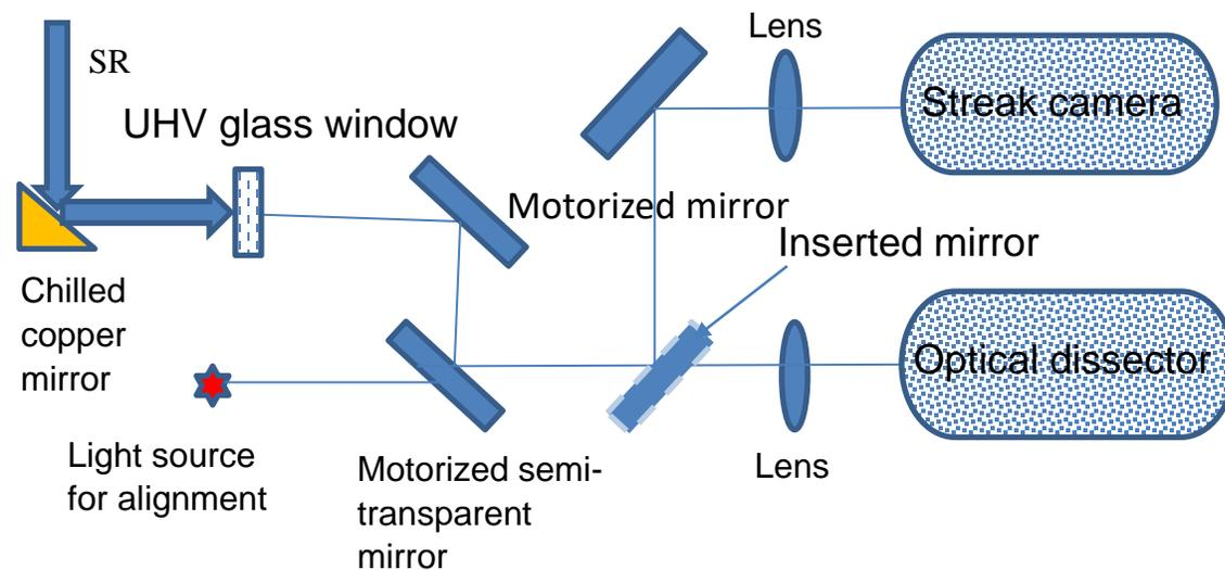
**Fig. 13.** Optical scheme of beam length measurements.
