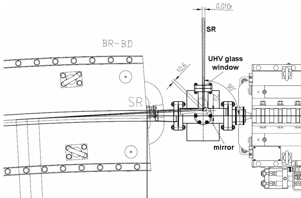
**Fig. 12.** Layout of one of the SR outlet.
