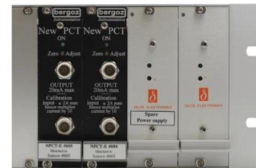
**Fig.7.** DCCTs from Bergoz with analog electronics.
