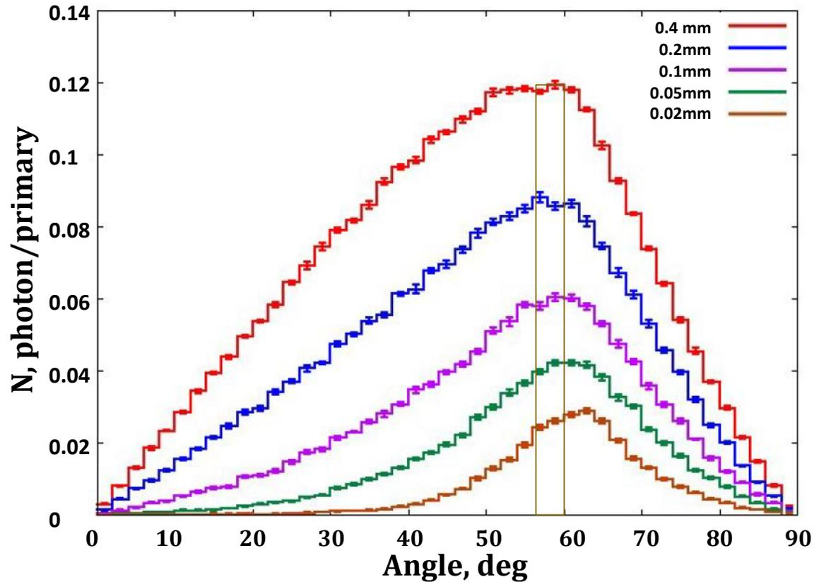
Cherenkov radiation angular distribution of **0.6 MeV** electrons beam through different quartz plate thicknesses.
