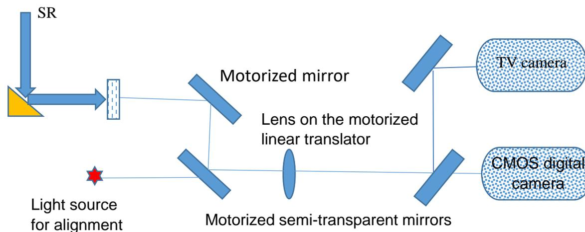
**Fig. 14.** Optical scheme of beam transverse profile measurements.
