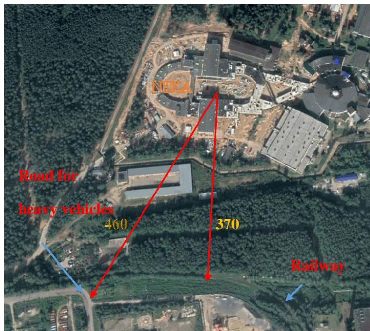
Fig. 13 Location of the NIKA collider relative to the main sources of microseismic noise (road and railways)
