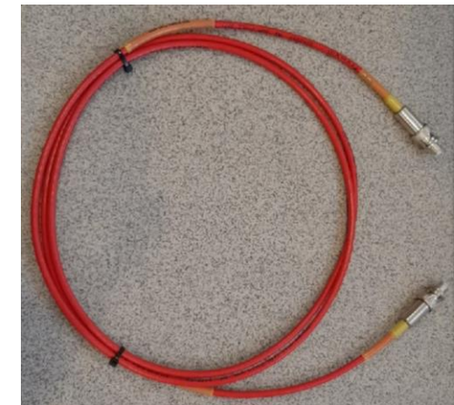
98 one core HV long cables with SHV connectors will be made directly in the MPD area
