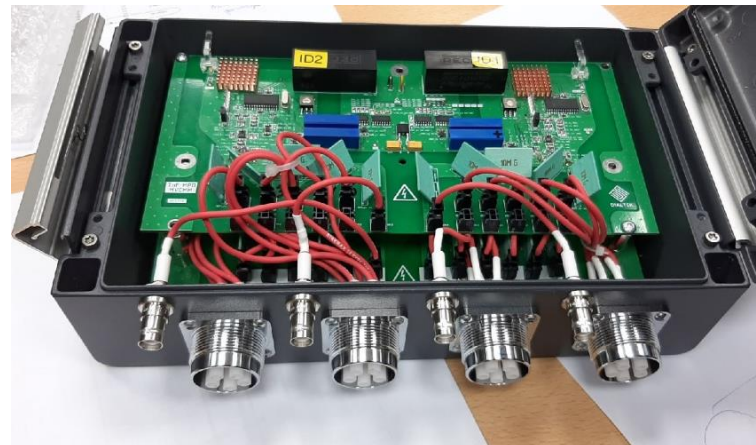
98 HV cables and 28 new distribution boxes for 28 TOF modules in production now
