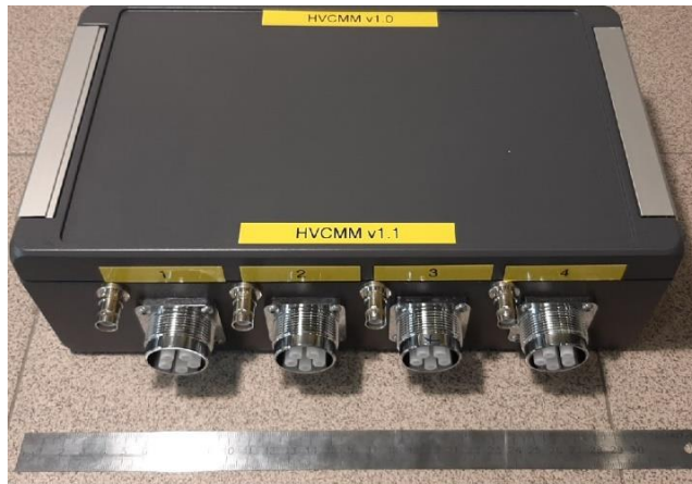
98 HV cables and 28 new distribution boxes for 28 TOF modules in production now
