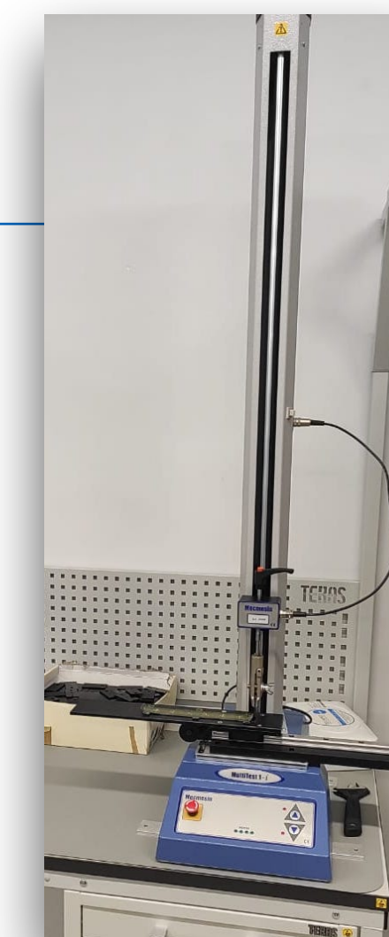
Peel test station
