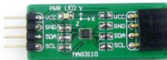
Figure 1 Mag3110 placed on a printed circuit board
