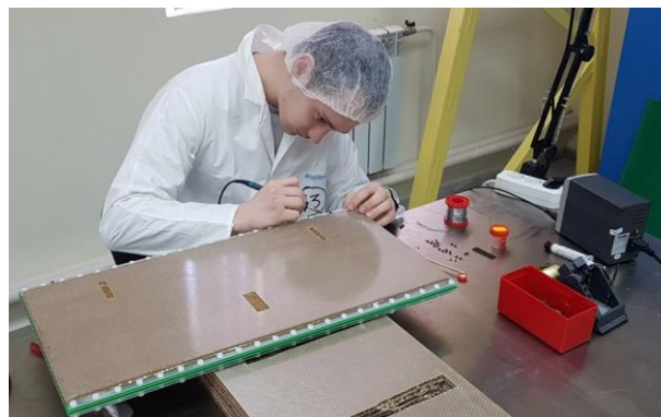
Soldering HV connector and readout pins
