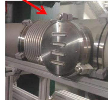
Four stainless steel vacuum boxes downstream the target are replaced by aluminum ones. The design and production of the target station control system and pneumatic actuator mechanics is performed by A.Kubankin group. Works to be finished by June 2021.
