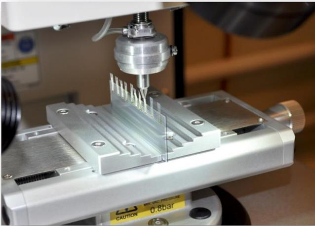
Mechanical testing of flexible cables during assembly
