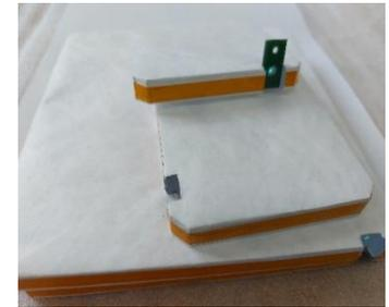
Light readout: MPPC Hamamatsu S14160-1310(1.3x1.3 mm<sup>2</sup>)
