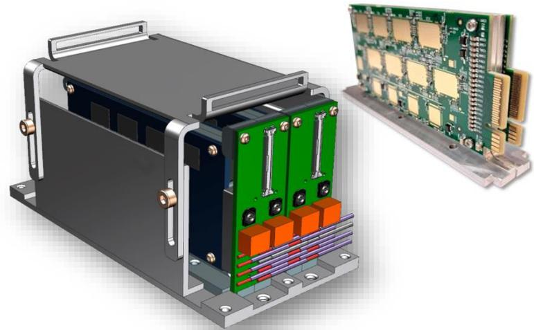
Custom-designed mechanical parts for the Front-end board
