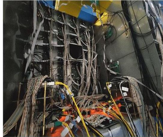
20 PSD CBM nodules - transverse size  $20 \times 20 \text{ cm}^2$ , 5.6 nuclear interaction lengths.
