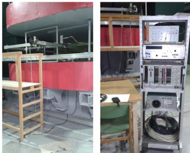
Figure: View to magnetic machine inside the SP-41 magnet control electronics and high precision current source
