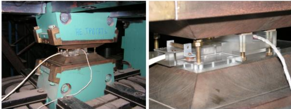
Figure: Calibration magnet up to 2 Tesla Plastic box for NMR-cell and Hall-sensor fastening
