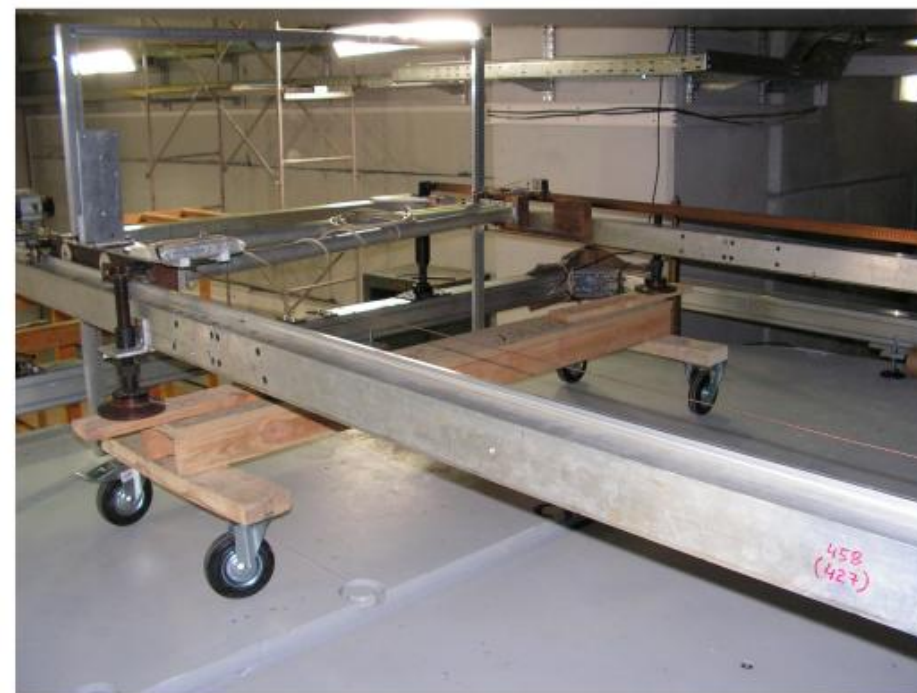
Figure: Magnetic machine inside the SP-41 and moving platform to change its position
