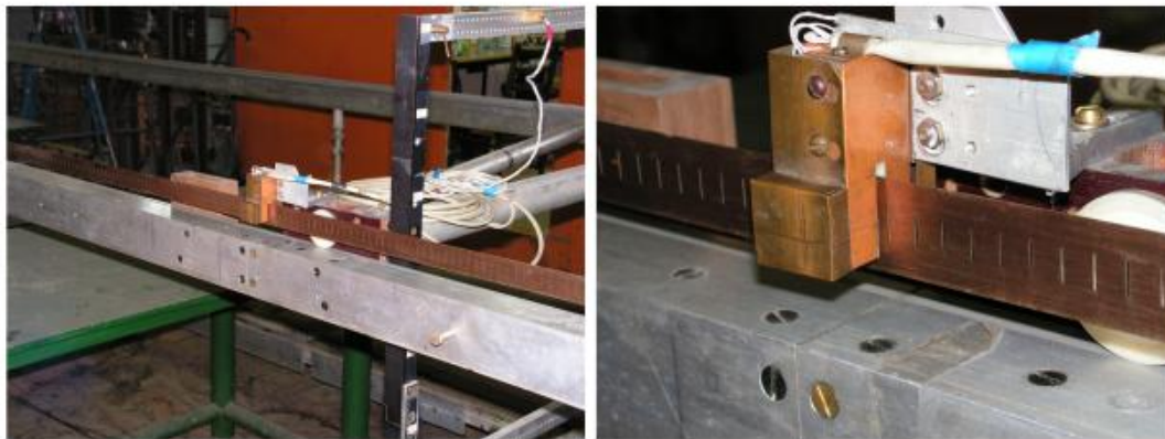
Figure: Trigger is generated by the LED-reader and perforated tape
