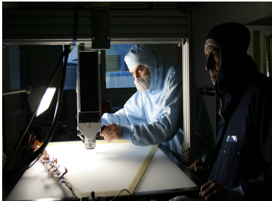
Figure 16: The repairing procedure of one of the Dubna MWDC-II sector at GSI.
