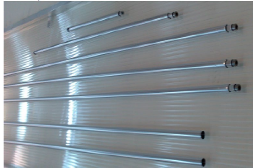
Fig.8 Sample tubes of 20 μm-thick walls with 70 nm-thick aluminum deposition.
