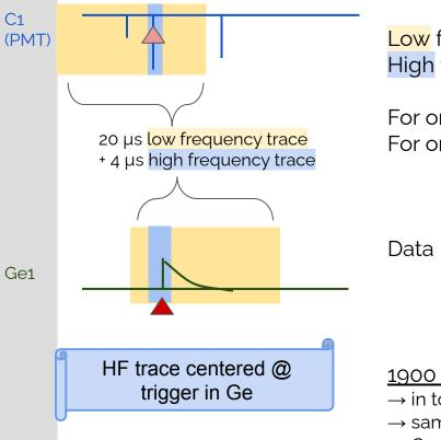
Low frequency trace: ~ 30 MHz | 600 samples | 1.2 kB High frequency trace: 125 MHz | 500 samples | 1 kB
