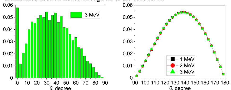
**Fig. 2-3.** The discrete probability densities of transmitted (on the left) and reflected (on the right) neutrons as functions of polar angle  $\theta$ , which is an angle between the incident and the scattered directions of a neutron.
