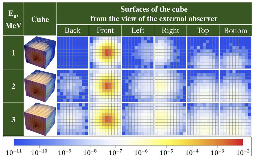
The thermalization of fast neutrons increases the probability of scattering and absorption during the propagation in the BPE media. As the result, the simulation confirms close to the isotropic angular distribution of the partly thermalized neutron fluxes through all of the cube faces.
