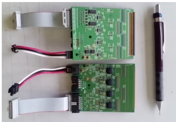
Fig. 3.3.3. 128 channel read-out board based on VA163 chip. Front and back side view.
