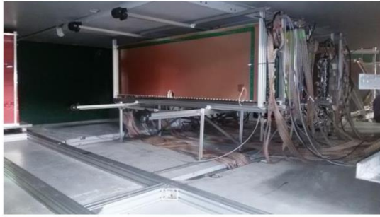
Figure 3.3.2. Left plot: GEM chambers integrated into BM@N experimental setup. Right plot: Cosmic ray test bench.
