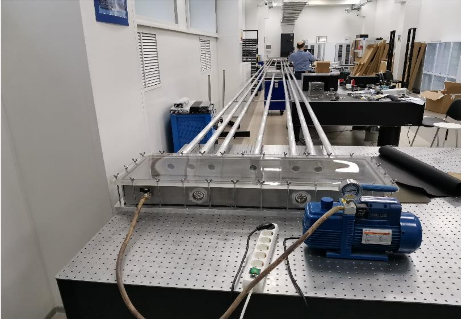
Laser Vacuum Reference Line 130m long at DLNP Metrological Laboratory
