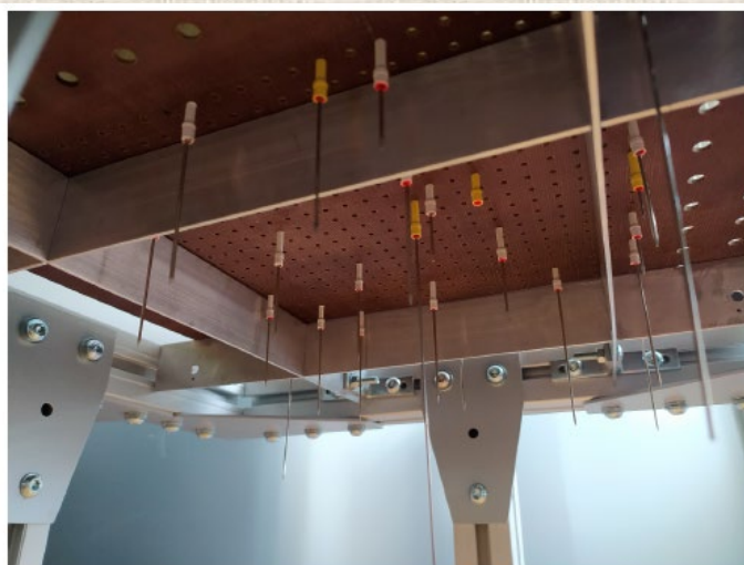
Fig. 3.2 - installing the spoke locks
