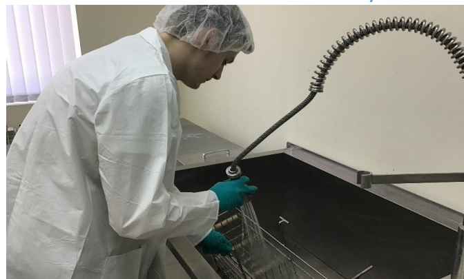
Glass cleaning with ultrasonic wave & deionized water
