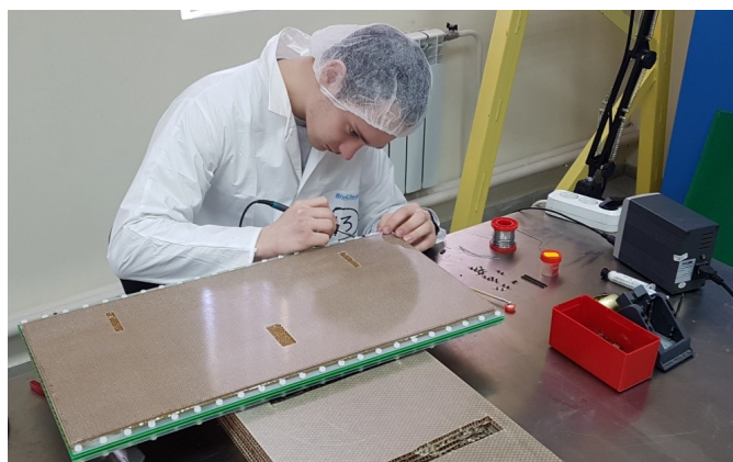
Soldering HV connector and readout pins
