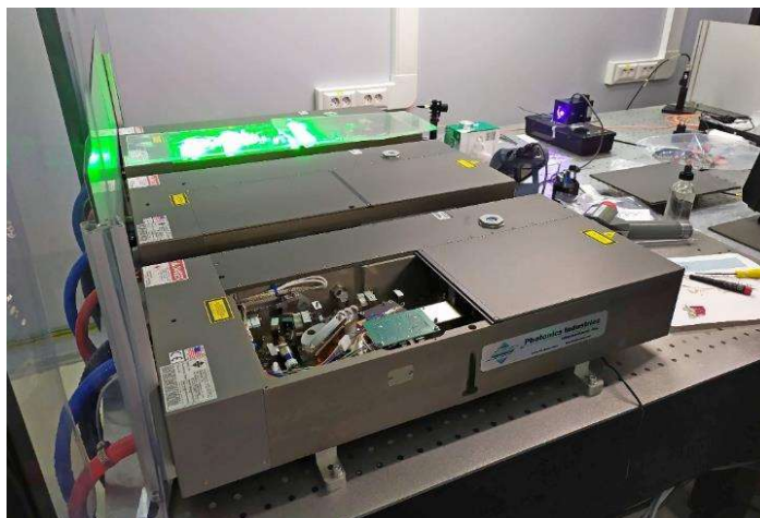
Fig. 18. Three new Photonic Industries TU-H Titanium-sapphire lasers installed in the GALS laser laboratory.
