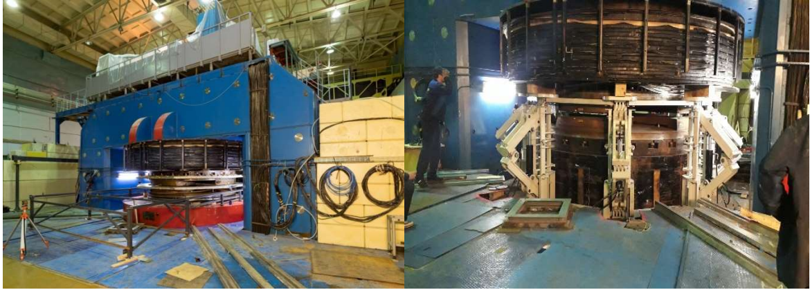
Fig. 5. Dismantling of the U400M main winding
