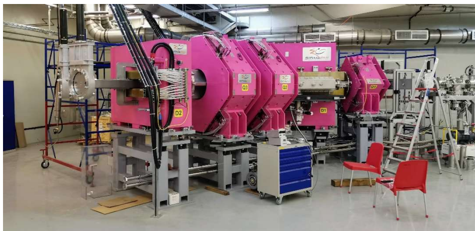
Fig. 14. Separator DGFS-3 (during assembly) at the experimental hall of the SHE Factory.
