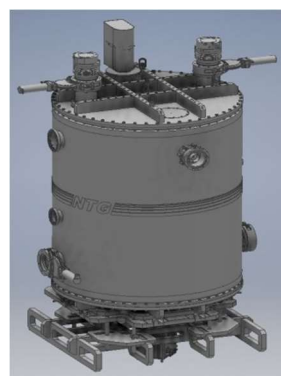
Fig. 11. The principal parameters and a side view of the RF kicker installed at the ACCULINNA-2 beam line after the achromatic focal plane F3.
