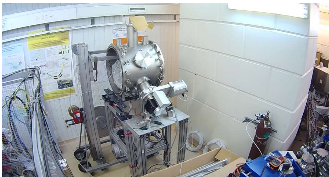
Fig. 16. Assembling of the cryogenic gas ion trap.
