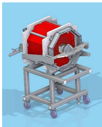
Fig. 5. Combined detection system SFiNX (116 He-3 neutron counters, 128x128 strips Micron-DSSSD). Efficiency for the single neutrons – 57%.
