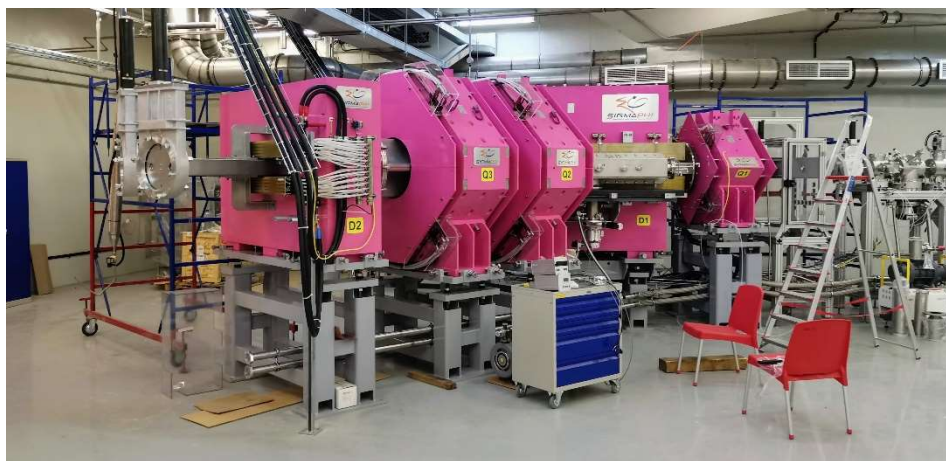
Fig. 2. Separator GFS-3 (during assembly) at the experimental hall of the SHE Factory.
