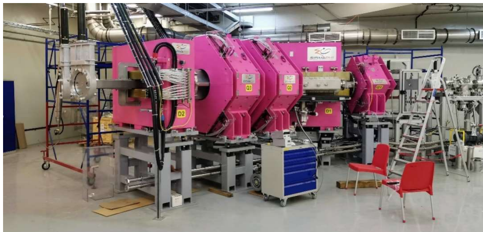
Fig. 13. Separator DGFS-3 (during assembly) at the experimental hall of the SHE Factory.
